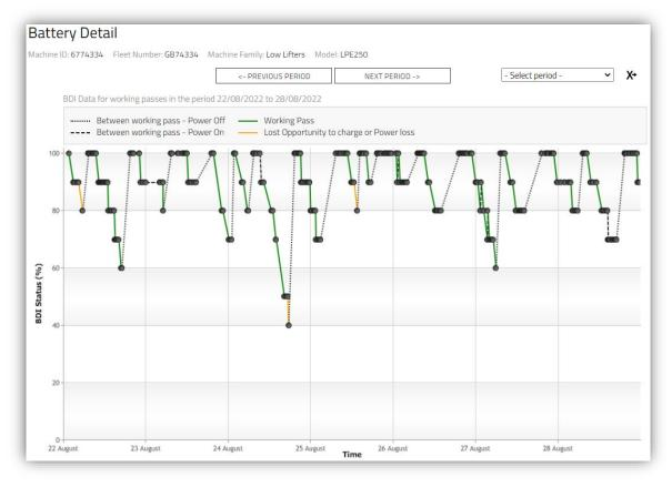
For **Li-lon batteries** you want to **oppurtunity charge** the truck whenever the truck is not in use, trying to keep the battery as full as possible inbetween usage.
