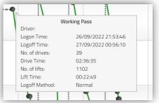
Please note CBIC trucks (Counter Balance Internal Combustion) with drivers who havn't logged off the truck before turning off the ignition of the truck will produce a Battery Disconnect error even though the truck doesn't have a battery.
